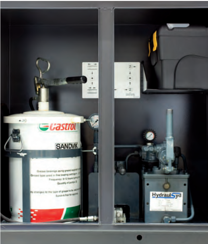
Fully enclosed hydraulic cabinet keeps dust and rain away
