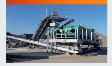
LOG WASHERS with a tub length up to 8,000 mm
